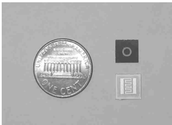
Fig. 5. The prototype of GaN gas sensor for alcohol detection with Pt heater on sapphire side presented on the right-down corner
